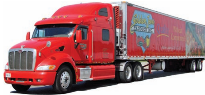
FIGURE 1-3 Tractor-trailer combination: a dual axle semi-trailer coupled to a 6 × 4 tractor. This is the most common rig observed on our highways
